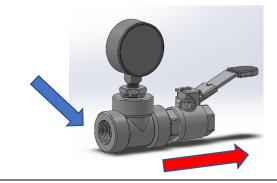
The open end (Green arrow) of the valve can be attached to a hose, or inline with the water supply, to measure inline flow pressure (valve open) or measure zero flow pressure (valve closed)
